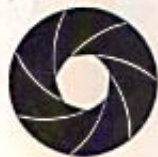
Lens at f/8 : Depth of field extended in front of/behind the main subject.
