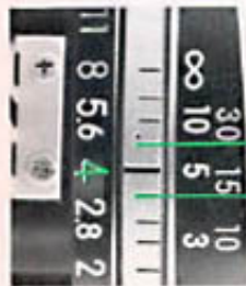
Lens set at f/4 : Shallow depth of field centered on the main subject.
