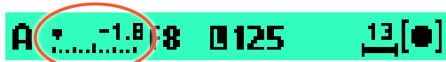
New metered area is 1.8 EV lower than the area metered when the AE-L button was pressed.
