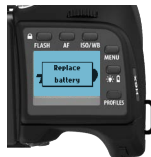
Exhausted battery warning
