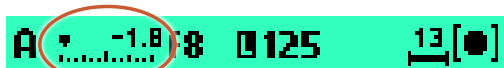
New metered area is 1.8 EV lower than the area metered when the AE-L button was pressed.
